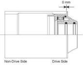
Put the Non-Drive Side Adapter (T) into the BB Shell (B).
