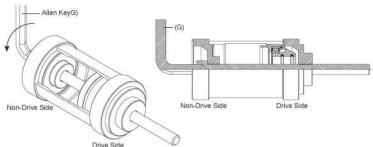
4.Remove the tool parts and have visual check to see if the Drive Side Adapter (A) was pressed to the correct position.
