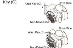
Clockwise tighten P220A (B) from two sides of the BB Shell (A) with two wrenches (D) at the same time (suggested torque: 46 Nm). Clockwise tighten the two bolts with the 4mm Allen Key (C) (suggested torque: 8.8 Nm).
