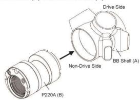
4. Clockwise tighten P220A (B) from both sides of the BB Shell (A) by hand and make sure both sides of P220A (B) are firmly close to the end surface of the BB Shell (A).
