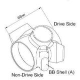
3. Fix the eccentric BB (B) by your palm to the end surface of the BB shell and make sure there is no gap in between.
