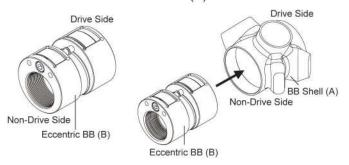
Clockwise tighten the screw with 5mm Allen key (C). (The suggested tightening torque is 18Nm.)
