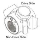
Make sure the direction of the eccentric BB (B) is correct. Install the drive side of the eccentric BB (B) into the non-drive side of the BB shell (A).
