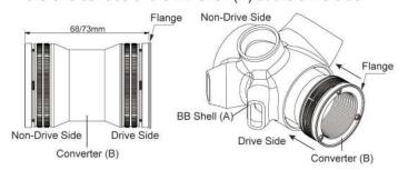
Slightly clockwise tighten the three bolts at the non-drive side with 2mm Allen key (C) separately. And then use the same way for the three bolts at the drive side. (Torque for Bolts: 2.1~2.3 Nm)
