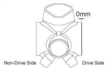
2. Make sure the direction of the converter (B) is correct. Install the converter (B) into the BB shell (A) from the drive side and lean the flange of the converter (B) against the end surface of the BB shell (A) at the drive side.
