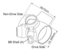
Fix the converter (B) by your palm to the end surface of the BB shell and make sure there is no gap in between.
