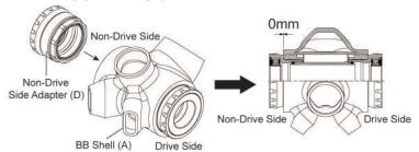
2. Counterclockwise tighten the Drive Side Adapter (B) with the Drive Side Converter (C) by hand.
