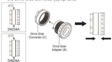
Follow step two and three to clockwise tighten the Non-Drive Side Adapter (D) and Non-Drive Side Converter (E). (The suggested tightening torque is 35~45 Nm.)
