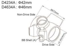
3. Counterclockwise tighten the adapter and converter with Open Wrench (38/40) and Shimano Wrench and make sure there is no gap in between. (The suggested tightening torque is 35~45 Nm.)
