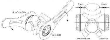
Clockwise turn the Non-Drive Side Adapter into the BB shell and manually tighten it together with the Drive Side Adapter.
