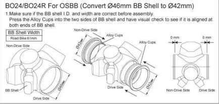
Use pressing tool to press the Drive-Side Adapter into the BB Shell. All actions should be aligned to the pressing area.
