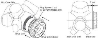
4.Tighten clockwise the Drive Side Adapter and the Non-Drive Side Adapter at the same time by wrenches.Remove the wrenches and have visual check to see if both the Drive Side Adapter and Non-Drive Side Adapter were pressed to the correct positions.
