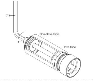
4. Tightly press the adapter with bearing (A) of R30, into the BB shell and stop the action till it leans against the Circlip (Q) . Have visual check to see if the adapter with bearing (A) was pressed to the correct position when removing the tools.
