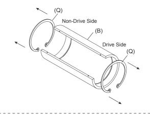
10.Disassembly is finished.
