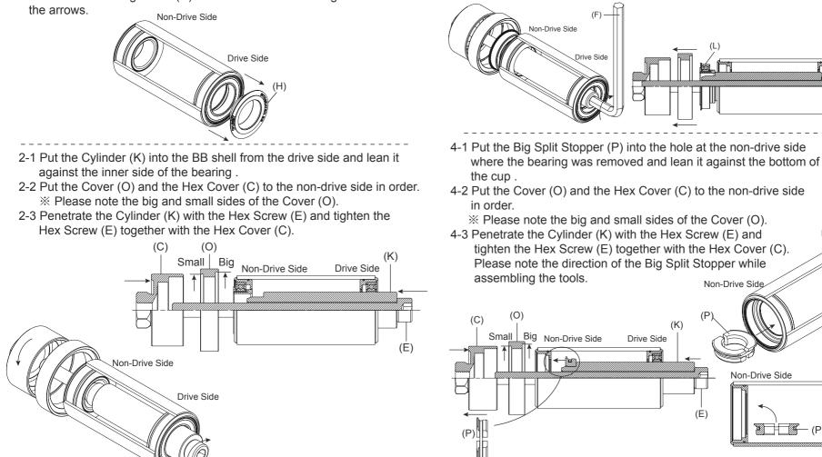
3. Tighten clockwisely the Hex Screw (E) by Allen Key (F)
