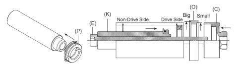
8.Tighten clockwisely the Hex Screw (E) by Allen Key (F) to take off the bearing (L) of the drive side.
