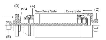
6.Tighten clockwisely the Hex Screw (E) by Allen Key (F).
