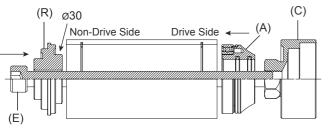
5.Penetrate the Hitch 22/24(D) with the Hex Screw (E)
